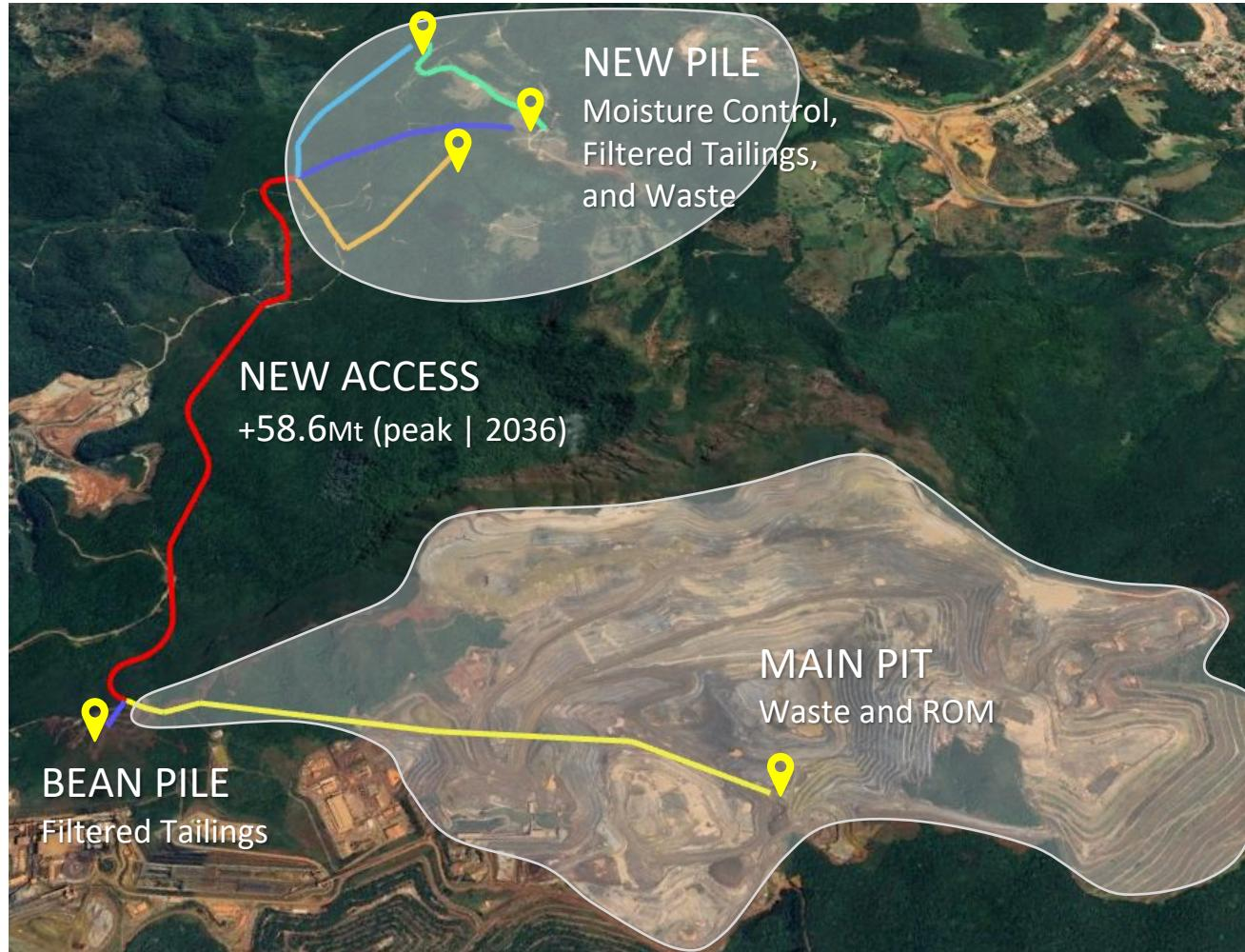
The mine operates 240-ton trucks. The hauled volume is expected to **DOUBLE** and will be dumped at a **NEW PILE** using an **EXCLUSIVE ACCESS**.
